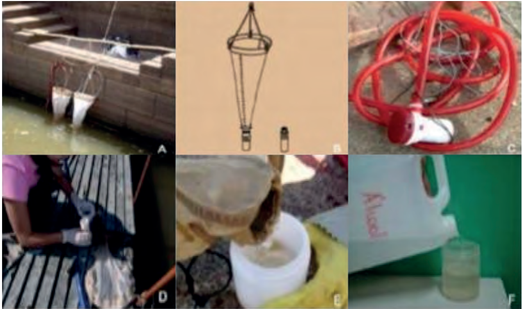
Figure 20. Collection of plankton samples for quantification of larvae of L. fortunei . A) filtration in plankton net, B) plankton net, C) suction pump, D and E) removal of the sample from the net and F) fixation of the sample in 80% alcohol. Source: Santos et al. (2012b).
