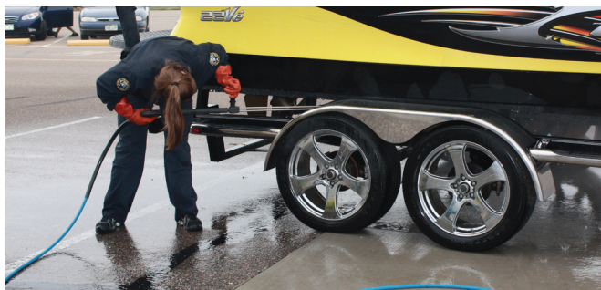
Watercraft inspection staff using hot water to decontaminate a boat. Photo courtesy of Elizabeth Brown, Colorado Parks and Wildlife.
