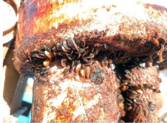
Golden mussels colonizing the exterior housing of water quality equipment at Rough and Ready Island in October 2024. Photo: Jay Aldrich (DWR)
