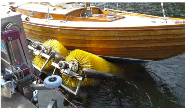
Figure 4.25 An example of a Boatwasher system cleaning the hull of a vessel. Source: www.boatwasher.wordpress.com .
