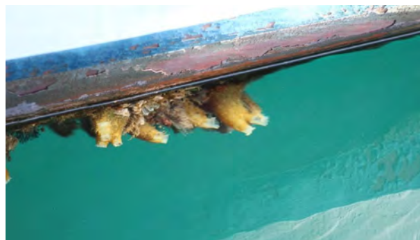
Figure 4.16 Biofouling by at least three invasive species ( Ciona robusta , Clavellina lepadiformis , Watersipora subtorquata ) on the hull of a recreational vessel with inefficient antifouling paint.
