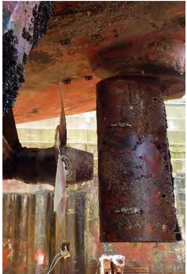
Figure A9 Niche areas: Rudders, hinges and rudder stock. Source: David Smith.
