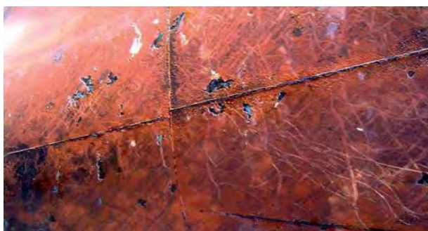
Figure 2.3. Ship's Hull showing pitting corrosion.
