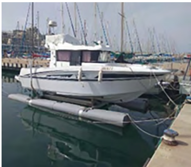
Figure 3.7 Example of an air berthing system.
