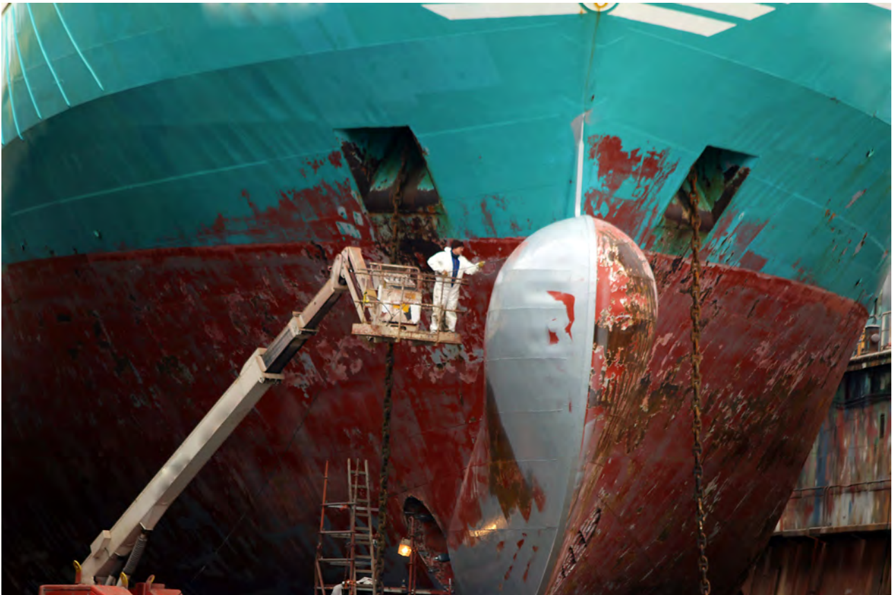
Figure 3.3 Applying an antifouling paint to a hull in a dry dock. Source: Lee Adamson.
