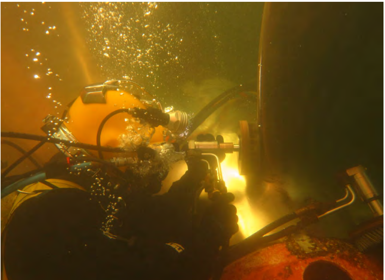
Figure 3.2 Diver undertaking propeller blade polishing in port. Source: Hydrex.
