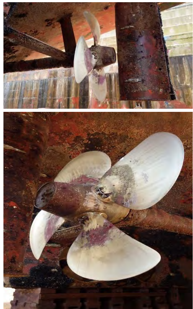
Figure A7 Niche areas: Propellers, shafts and struts. Source: David Smith.
