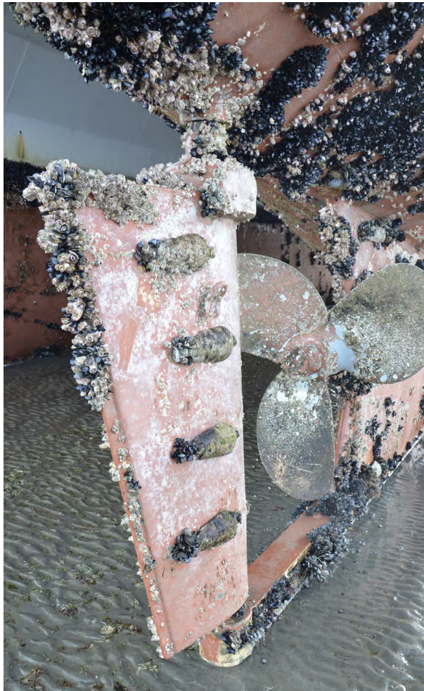
Figure 1.2 Macrofouling consisting of barnacles and mussels.
