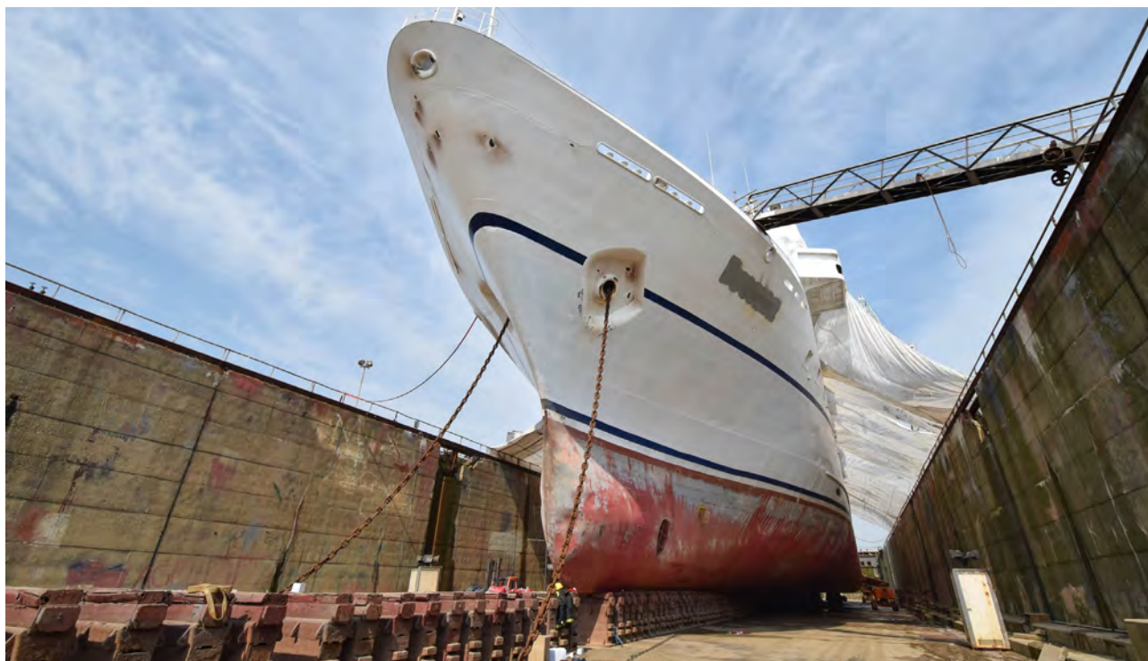
Figure 4.1 Vessels such as large passenger ships are designed for greater speed with above-water accommodation and amenity spaces and thus have a comparatively shallow operating draft when loaded and a small WSA.
