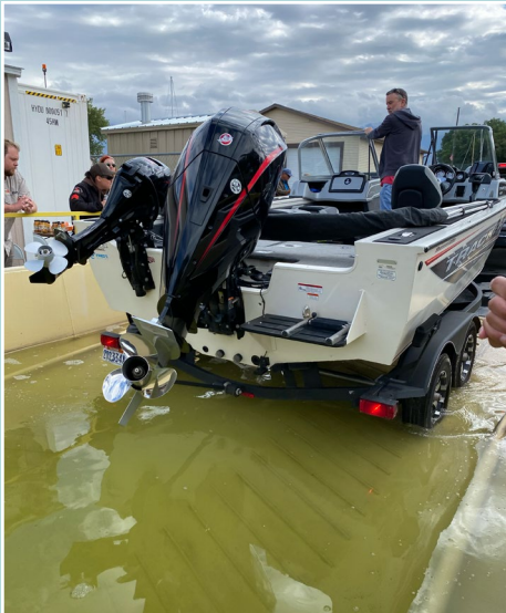
Two dip tanks in Utah. Left: Watercraft entering the dip tank on a traction ramp at Utah Lake. Below: Tank with hot water ready for watercraft decontamination at Sand Hollow. Photo credit: Clean Wake, LLC.
