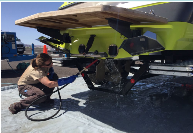
Figure 1. Operational variations of decontamination units. Top left: Mobile trailered unit. Bottom left: Recycled water circulating decontamination system. Above right: Mobile unit coupled with movable water collection tarp (photo: Quagga D, LLC).
